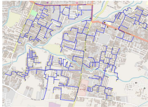
Figure 6. MST result using Borůvka's algorithm: illustrating the convergence of component-based merging into a single optimal spanning tree.
